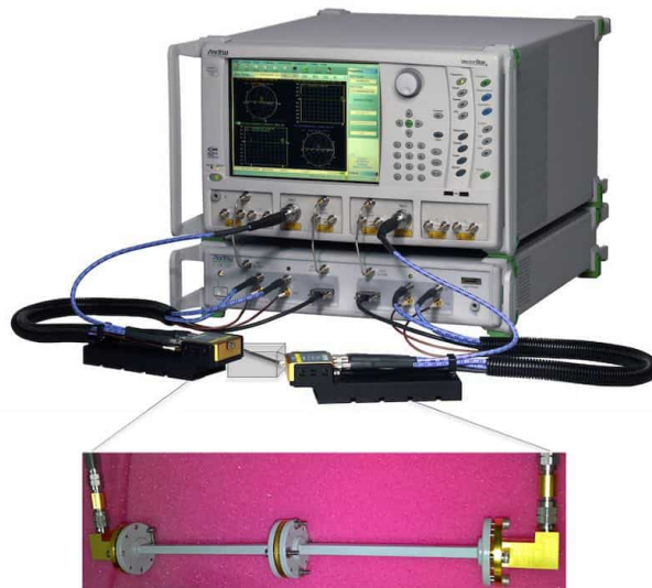
FIGURE 1.1 – Ligne de transmission (source internet : RF & Microwave Material Measurements: Techniques and Applications).
